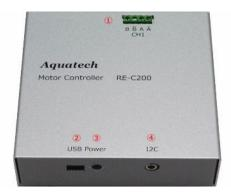
Motor connection terminals (CH1): B/B /A/A
